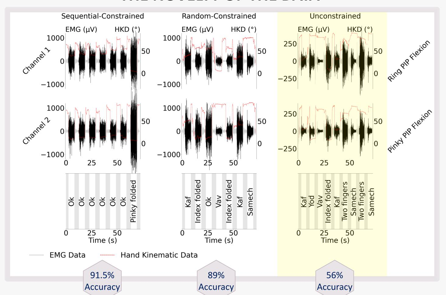
**Figure 1**. sEMG and hand-kinematic signals during unconstrained gestures (left) and during force-plus-rest instructions delivered in random (middle) or sequential (right) order. Black solid lines are sEMG signals from two electrode channels; red dashed lines overlay the corresponding joint-angle trajectories. Dark horizontal bands mark the active gesture periods, and gray regions indicate transitions.
